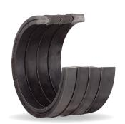
Merkel V-Packing Set V1000 is used for sealing piston rods, plungers and, in exceptional cases, pistons in highly demanding heavy industry applications. Each set comprises of one pressure ring, three or four V-packing rings and one support ring. A V1000 set is supplied either without back rings or with one or alternatively with two back rings at the support ring for enhanced extrusion resistance.
