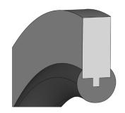
Fastener seals consist of an inner rubber component used in conjunction with an outer metal washer that supports the sealing functionality of applications such as screws or bolts. The rubber and metal combination creates an ideal fit to eliminate any clearance gaps between the housing components and protects against potential leaks in many static applications.
