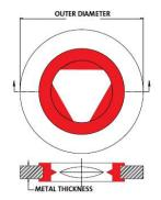
This diagram is a general guideline for how to measure the outer diameter (OD) and inner diameter (ID) of USZL seals
