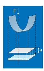
P = Permissible surface pressure [N/mm<sup>2</sup>] d = Rod diameter (rod guide) resp. piston diameter (piston guide) [mm]
