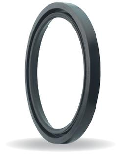
Merkel Radiamatic R35 is a radial shaft seal consisting of a fabric reinforced section of sturdy design, firmly bonded to the rubber sealing lip. A garter spring assists radial contact pressure of the lip on the shaft.
