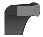
Our Dichtomatik brand NuPac is a precision-molded seal combining a U-cup with an O-ring. Under zero and low pressure, the O-ring pressurizes the lips of the U-cup allowing it to properly seal. As system pressure increases, the O-ring is energized and forces the lips outward, changing its behavior from a squeeze-type seal to a traditional lip seal. The NuPac is suitable for temperatures between -40°F and 212°F (-40°C to 100°C) and pressures from zero to 6,000 PSI.
