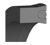
Our Dichtomatik brand NuPac is a precision-molded seal combining a U-cup with an O-ring. Under zero and low pressure, the O-ring pressurizes the lips of the U-cup allowing it to properly seal. As system pressure increases, the O-ring is energized and forces the lips outward, changing its behavior from a squeeze-type seal to a traditional lip seal. The NuPac is suitable for temperatures between -40°F and 212°F (-40°C to 100°C) and pressures from zero to 6,000 PSI.
