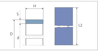
Calculating stretched length L2 for rods / pistons: L2 =  $(D - S) \times 3,11 - 0,5$  / L2 =  $(d + S) \times 3,11 - 0,5$
