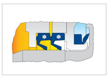
Sealing system featuring a Merkel Radiamatic RPM41 rotary shaft seal and an Merkel Enviromatic EA deflector for grease-lubricated bearings and cover plated housings.
