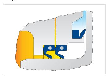
Sealing system featuring a Merkel Radiamatic RPM41 rotary shaft seal and an Merkel Enviromatic EA deflector for grease-lubricated bearings and open housings.
