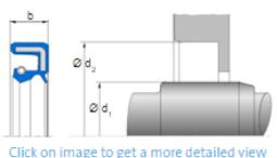
Inner diameter (d<sub>1</sub>): 68 mm
